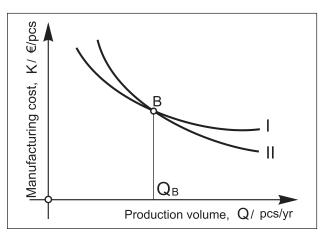
Figure 6 Diagram of the total manufacturing costs per product unit, for two blank variants [13]
