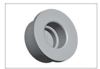
Figure 2 Group blank manufactured by cold bulk forming
