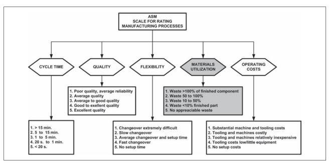
Figure 4 Parameters of manufacturing process in the metalworking industry (Rating: 1-poorest; 5-best) [9]
