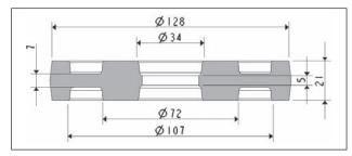
Figure 5 Group forging for the gear group from Table 1
