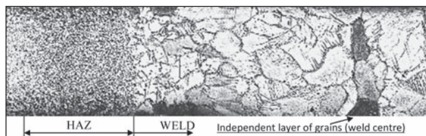
Figure 7 Macrograph of a part of BWJ with a layer of independent grains in weld centre; 1 mm thick FSS, I = 40 A, V = 0,31 m/min, U = 12 V, gas: Ar + 5 % H 2
