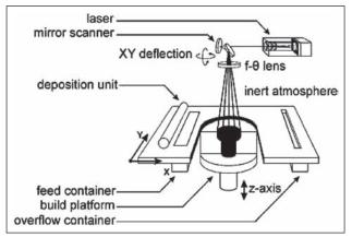
Figure 2 Principle of the SLM [18]
