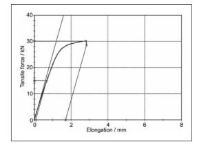
Figure 5 Tensile curve for specimen No. 1
