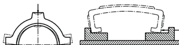
Figure 1 Deformation of a work piece during clamping Slika 1. Deformacija radnog komada kod stezanja
