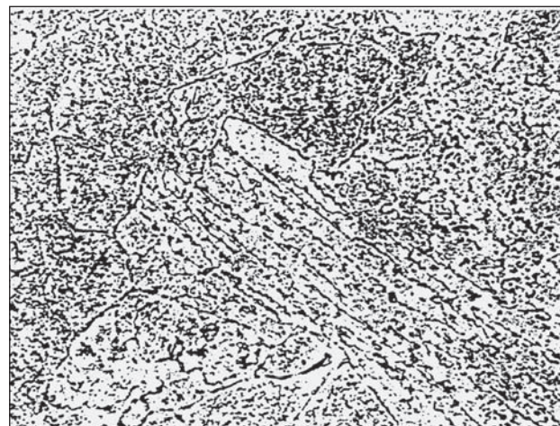
Figure 5 Microstructure of tested steel after 1,57 \cdot 10^5 h in service, magn. 800x
