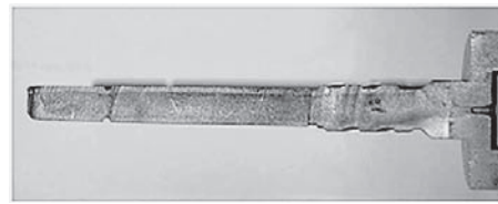
Figure 6 Heat treated planetary shaft - longitudinal cross-section
