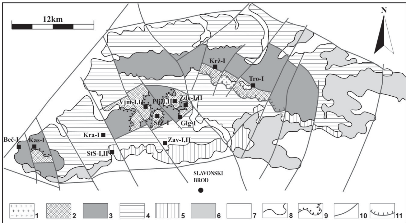
Figure 3: Geological sketch map of Dilj gora Mt. (simplified from the Basic Geological Map of Croatia 1:300000; CROATIAN GEOLOGICAL SURVEY, 2009) with locations of the studied sections. Legend: 1 – magmatic rocks; 2 – Badenian; 3 – Sarmatian + Pannonian; 4 – Pontian; 5 – Pliocene; 6 – Pleistocene; 7 – Holocene; 8 – normal boundary; 9 – transgressive boundary; 10 – fault; 11 – thrust.
