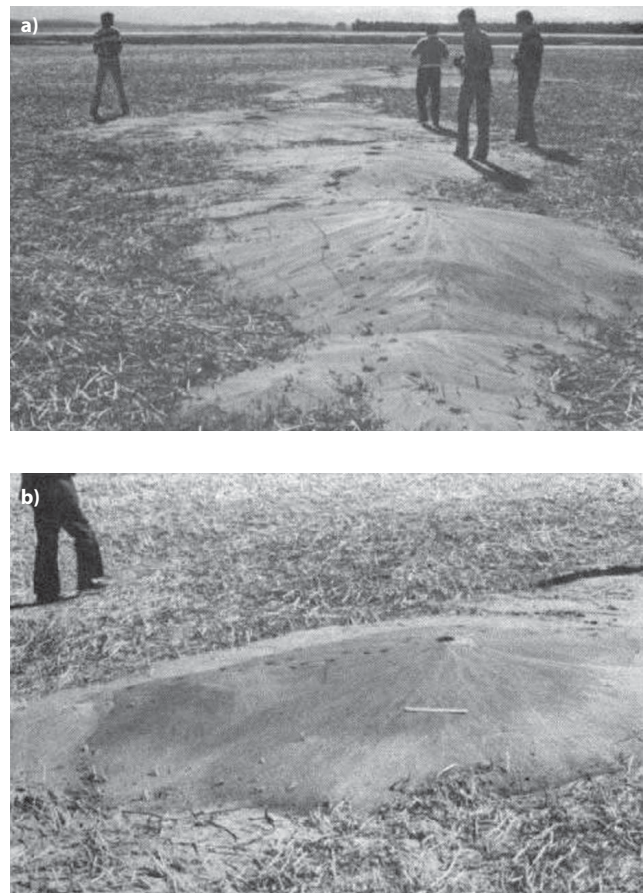
Figure 4: Craters of liquefied soil on banks of the River Chlef (a and b).
