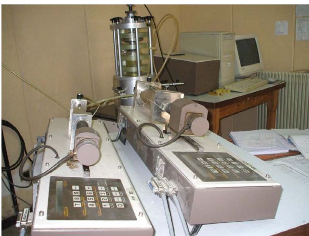
Figure 7: The triaxial system set up.
