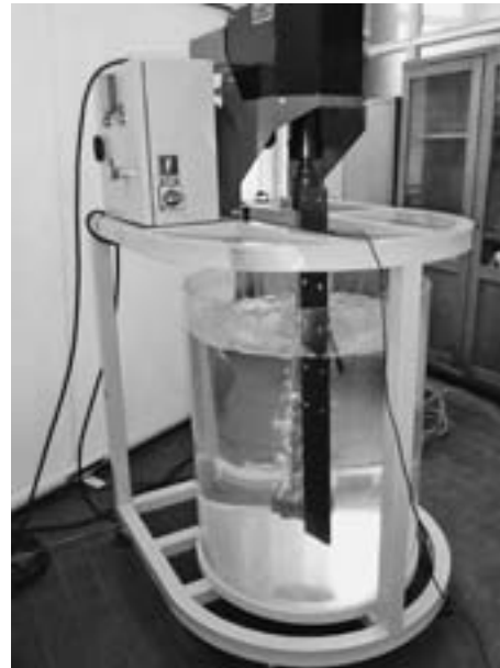
Figure 3 The view of test stand for the modelling research in the URO-200 reactor
