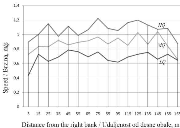
Figure 4. The dependency of the partial speeds of the transversal section of the River Drava watercourse to the distance from the riverbank for three various water levels, measuring station Donji Miholjac
