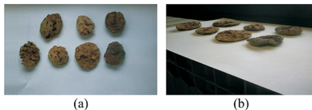
Figure 4 Formed replicas of the largest damages at the bottom of the boiler RP7; (a) The top view: Upper row - Damages at the left hand side end of flange; Lower row - Damages at the right hand side end of flange; (b) The side view
