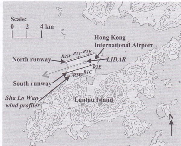
**Figure 1.** Map of Hong Kong International Airport and the adjacent areas (height contours: 100 m). Equipment labels are in italic fonts. Black dots are the airfield anemometers. The grey arrow is the viewing direction of the staring LIDAR beam.
