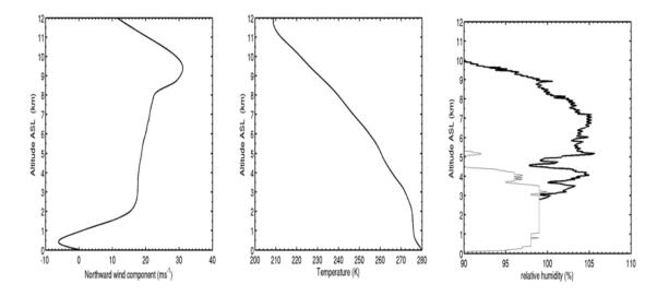
Figure 1 Left: interpolated northward component of the background wind profile. Center: interpolated background temperature profile. Right: relative humidity profiles measured over water from radiosounding (thin line) and evaluated over ice (bold line).
