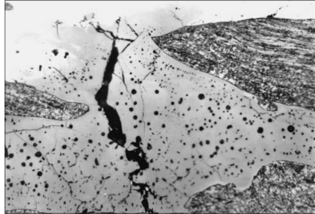
Figure 8 Annealed sample microstructure (450 °C through 6 hours), Magnification 400 ×
