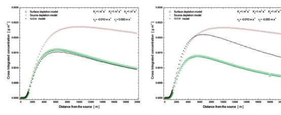
Figure 1. CIC at a ground level for the three models with  $v_d$ =-0.010 ms<sup>-1</sup> and  $v_s$ =0.0 ms<sup>-1</sup>
