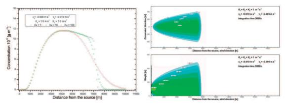
Figure 3. Left: ground level concentration above the plume center line for different  $K_x$ . Right-upper: ground level concentration. Right-lower (x,z) at the plume center line direction.
