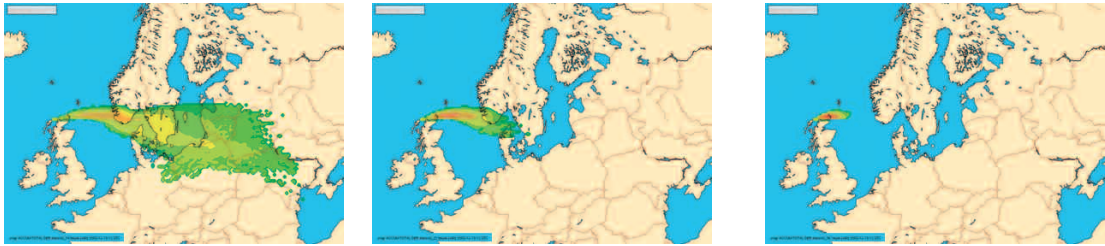
Figure 2. Accumulated total deposition for class 4 (left), 5 (middle) and 6 (right) of the particle radius, 60 hours after explosion.
