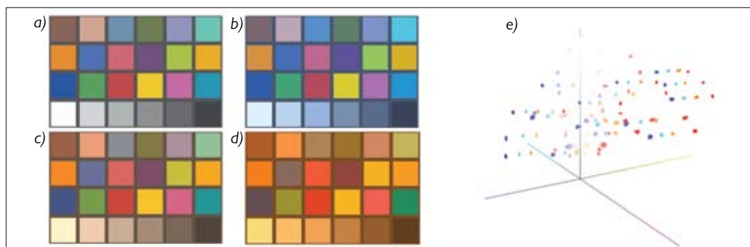
Figure 2: a) Original image with assigned profile with gamma value of 1.8 (D50 - 5000K) Simulated images after changing illuminant to b) D65-6500K, c) F11-4000K d) A-2856K. e) Colour gamut of initial and simulated images shown in the CIE Lab space (2a: cyan, 2b: blue, 2c: yellow, 2d: red)
