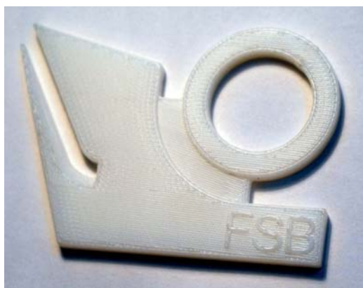
SLIKA 4 - Prototip otvarača za pisma načinjen postupkom FDM FIGURE 4 - Letter opener prototype made by FDM process
