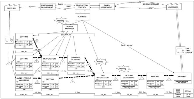
Figure 4 Current Value stream map of high-voltage pylons production Slika 4. Mapa trenutnog stanja proizvodnje dalekovodnih stupova
