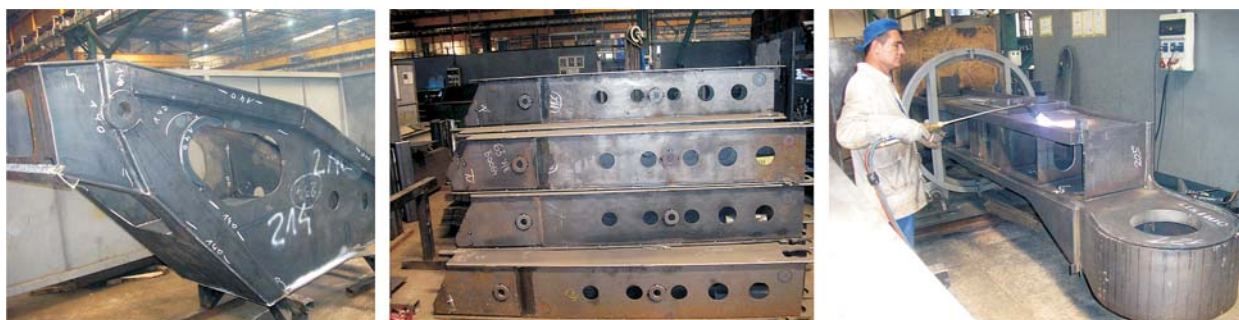
Figure 1 Welded structure forms made of S 960 QL steel where cracks appeared Slika 1. Zavarene konstrukcije od čelika S 960 QL s uobičajenim pukotinama
