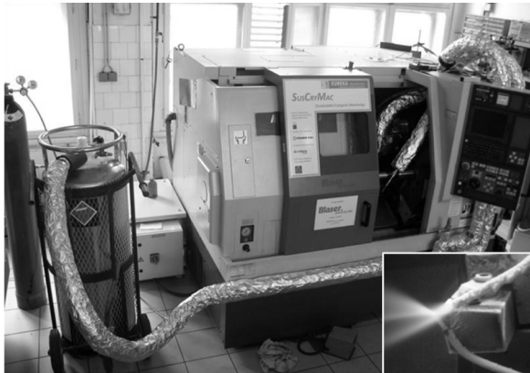
Figure 3. Cryogenic machining set-up with cryogenic fluid (LN) delivery into the cutting zone
