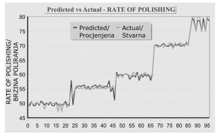
**Figure 3.** Presentation of actual and predicted values given by NN for the rate of polishing
