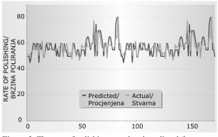
**Figure 2.** The rate of polishing actual and predicted (by a mathematical model (15)) values
