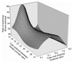
**Figure 1.** Functional dependence of the rate of polishing on outside diameter and oval shape of the tube
