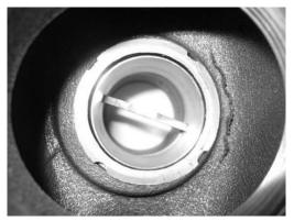
Figure 15. Problems of CNC machining due to valve opening not being coaxial
