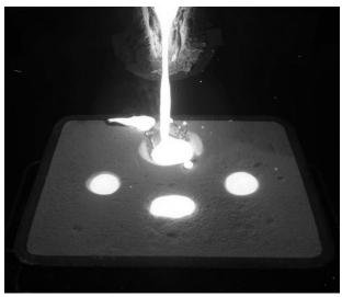
Figure 10. Grey cast iron casting into a finished form. Casting is completed once the melt pours out of the feeder openings
