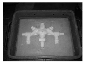
**Figure 4.** Form preparation starts with placing of one half of the pattern into the steel frame
