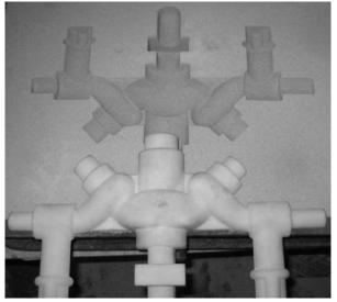
**Figure 7.** Cured sand form, with plastic pattern already removed. Other form half was manufactured in a similar manner.
