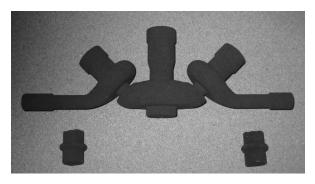
**Figure 8.** Sand cores made with Generis Sand Process on S 15 machine.
