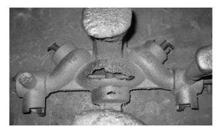
Figure 12. Hole in the casting, caused by lifting of the broken core
