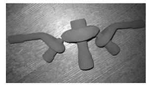
Figure 13. Core breaking on part with smallest core thickness Slika 13. Jedro ventila slomilo se na području najmanje debljine jedra
