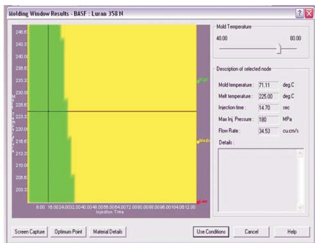
Figure 4 Mold temperature, Melting temperature, Injection time, Max. injection pressure, Flow rate. The stated results have been obtained based on the dimensions of the gear wheel, i.e. the chosen place for the injecting nozzle
