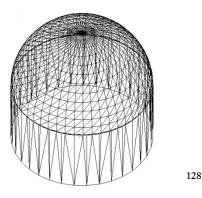
Composing the object from a high number of triangles will make the facets so small that the 3D printer is incapable of printing them "accurately" and the resultant physical object is actually rounded as the designer intended.<sup>129</sup>
