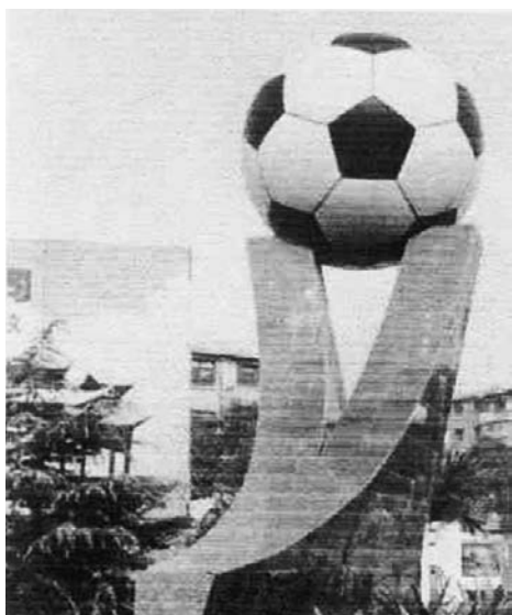
Figure 10 Hydrobulged steel football of 4000 mm diameter [10]
