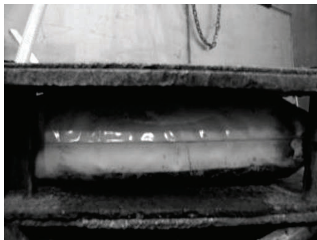
Figure 4 Schematic presentation of the experimental set-up for double hull construction, outer hull 14-19 mm thick, inner hull 12-14 mm thick
