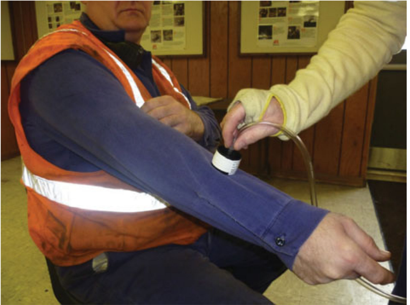
FIGURE 2. Vacuum sampling on an employee's uniform sleeve after removing cut-resistant sleeve. (color figure available online)
