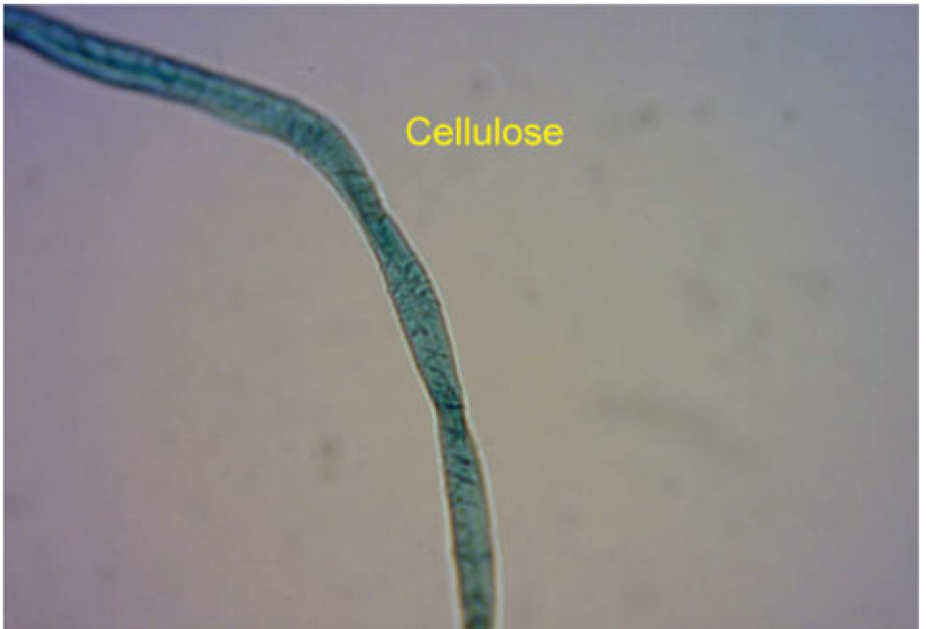
FIGURE 6. Photomicrograph showing cellulose on sleeve at 200 \times . (color figure available online)
