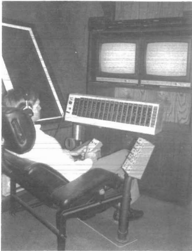
Figure 4.—Ergonomically designed workstation for teleoperator. (Photo by William H. Lewis, Pittsburgh Research Center.)
