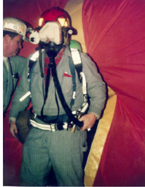
Figure 7 - A rescue team member wearing the Cairns IRIS and exiting a smoke-filled entry.
