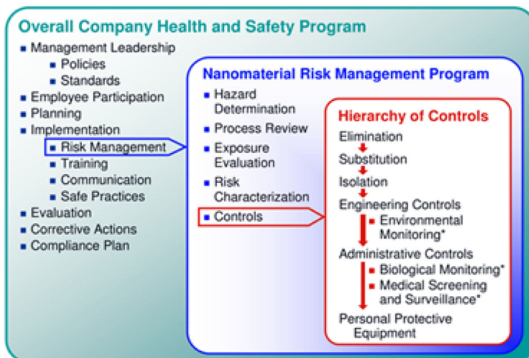
Figure 5. Components of an overall health and safety program that includes nanomaterial risk management (Schulte et al. , 2008).
