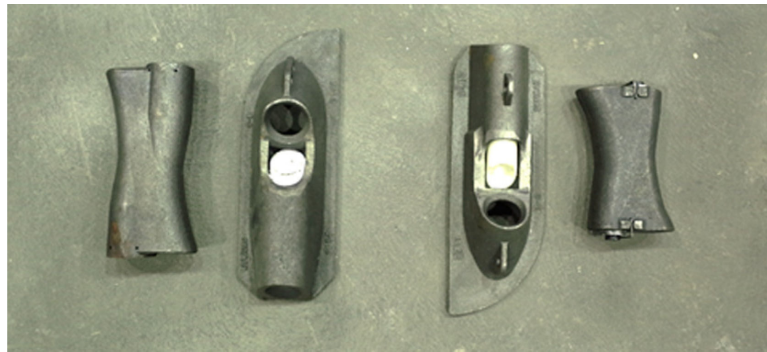
Fig. 3. Shoes and dog bones for 17 mm cable (l) and 15 mm cable (r).
