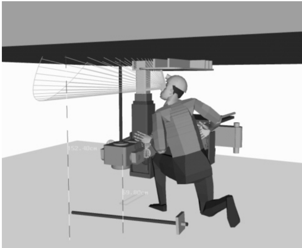
Figure 2b. Operator's risk behavior, hand on boom arm.
