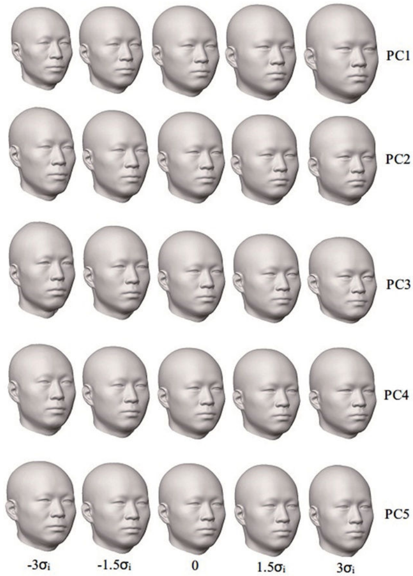
Figure 5. Male shape variations along the first five principal components (from left to right are reconstructed shapes at -3\sigma_j , -1.5\sigma_j , 0 , 1.5\sigma_j , and 3\sigma_j , j = 1, \dots, 5 ).
