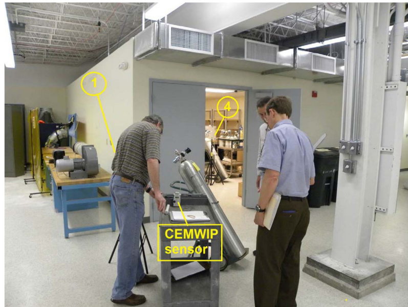
FIGURE 3. The NIOSH ventilation laboratory, staged with two standard gas cylinders at locations 1 and 4, with a tagged sensor on a mobile cart ready for experiment.
