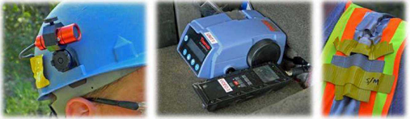
Fig. 1. (From left to right ) video camera attached to helmet, dust monitor and video monitor, and safety vest to hold instrumentation
