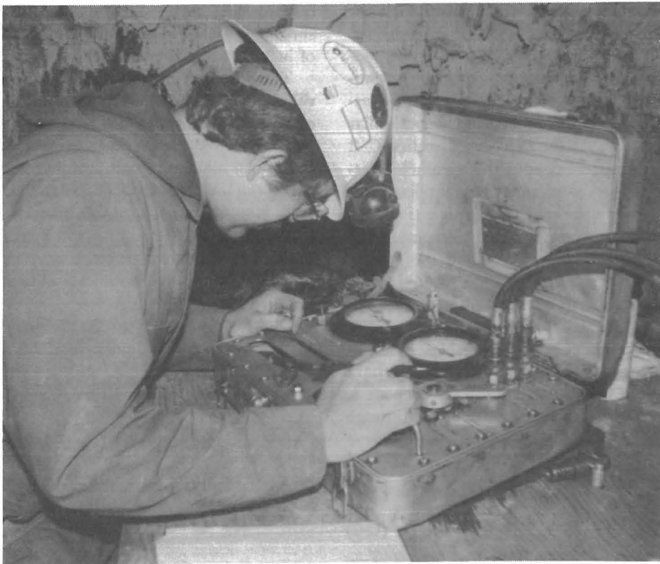
Figure B-7.—Borehole shear tester (BST). Top, installation in roof borehole; bottom, control console.
