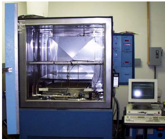
Figure 8. Guarded Sweating Hot Plate in Environmental Chamber
