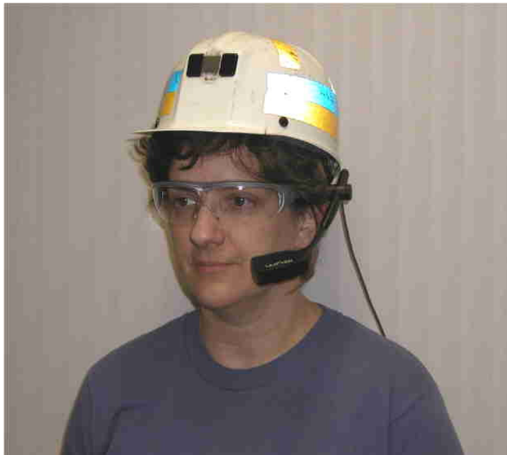
Figure 12.—The M920-CF does not obstruct the user’s frontal or peripheral line of sight.
