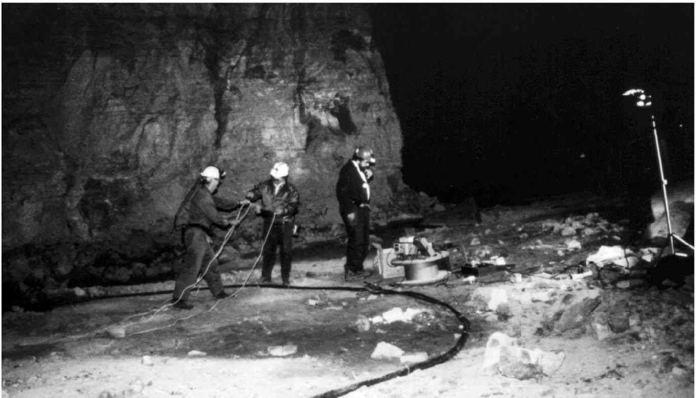
Figure 5.—A previous 7.5-m loop antenna in old workings of Lake Lynn mine site.
