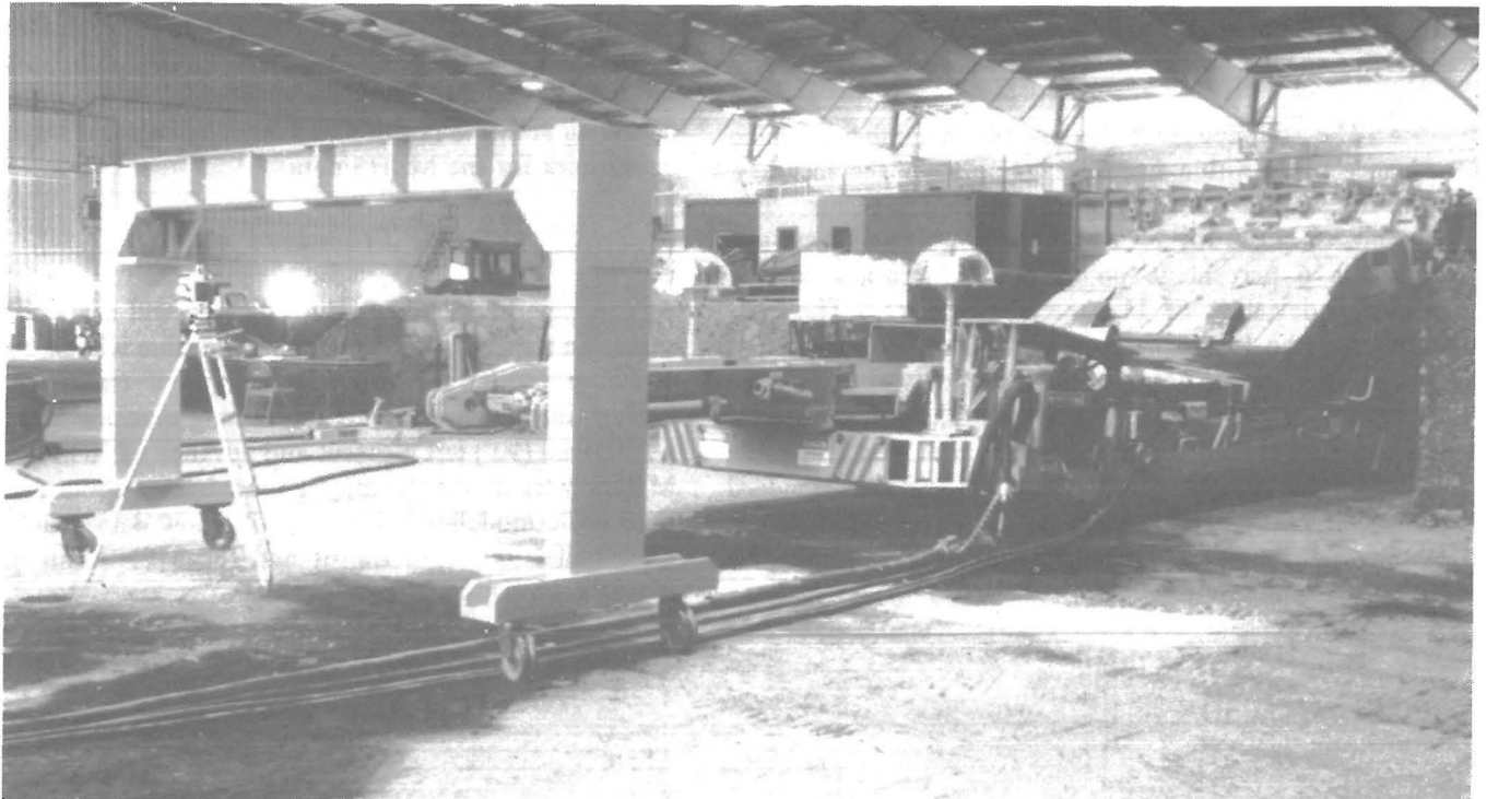
Figure 17.—Joy 14CM mining machine configured for MPHS surface tests.
