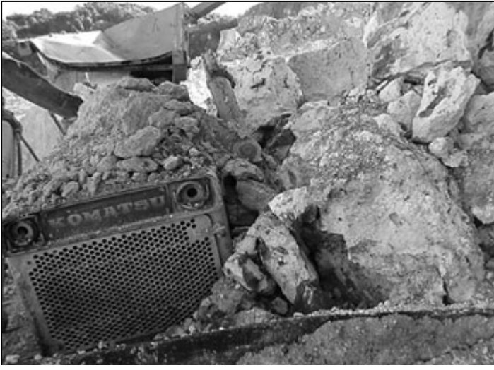
Figure 1.—Highwall failure at a stone operation crushed dozer and fatally injured dozer operator (November 13, 2002). (Photograph courtesy of Mine Safety and Health Administration, 2002.)
