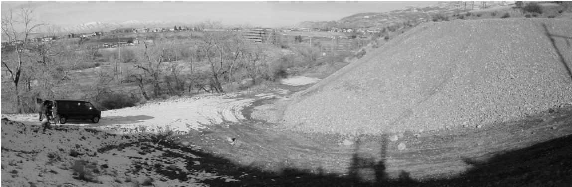
Figure 7.—Site of YINSAR slope monitoring experiments. Gravel pile is about 11 m high and has a slope of about 35^\circ .
