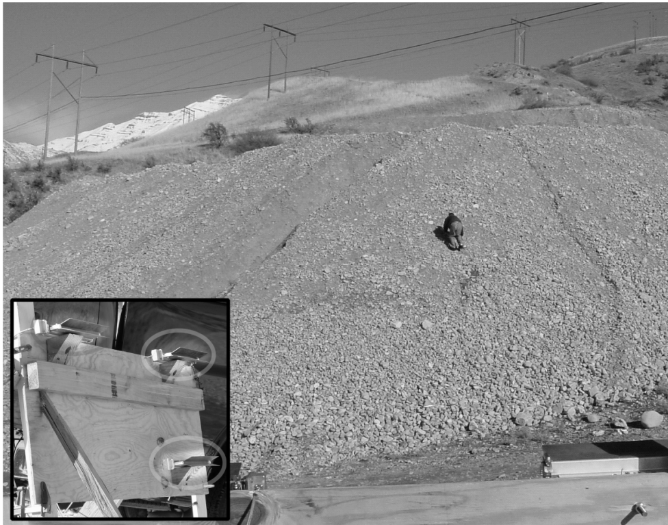
Figure 8.—Radar view of slope with man climbing. Inset shows transmitting antenna (left highlight) and receiving antennas (right highlights).
