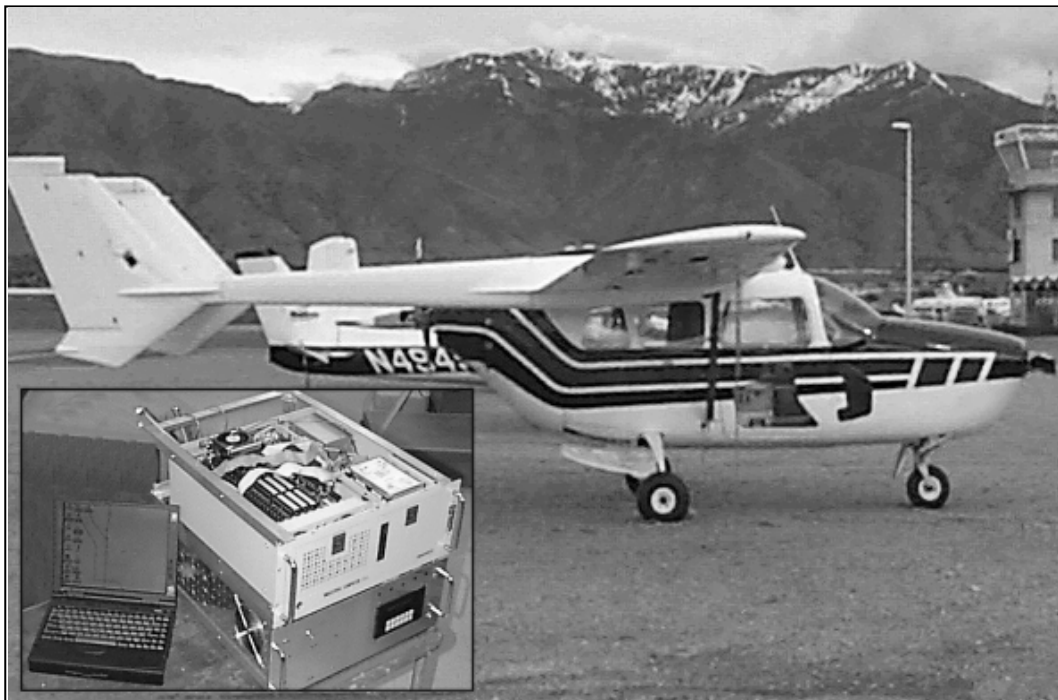
Figure 3.—Aircraft carrying the InSAR system. Insert shows computer and IF/RF subsystems, and laptop controller.
