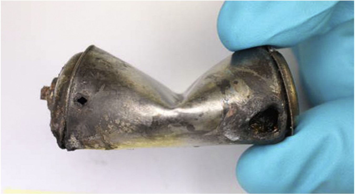
Fig. 6. An M52EX cell crushed by the plastic wedge that ignited the chamber atmosphere with two holes burned through the side of the cell can.
