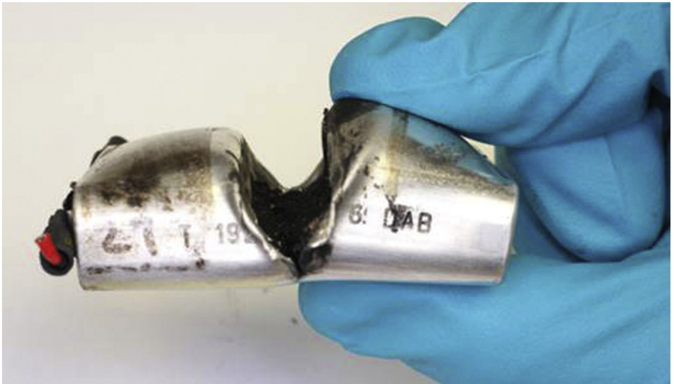
Fig. 5. An MP cell crushed by the plastic wedge at a slower speed that produced a lower overpressure thermal event. The cell swelled significantly.
