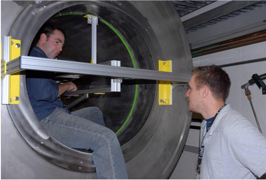
Figure 1. Western Michigan University students Jonathon Lighthall (left) and Jack Winkelbauer (right) mapping the field of the HELIOS magnet.
