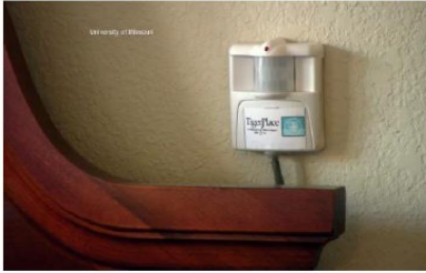
4) Also, wall sensor detects Joan falling by recognizing her heart rates acceleration
