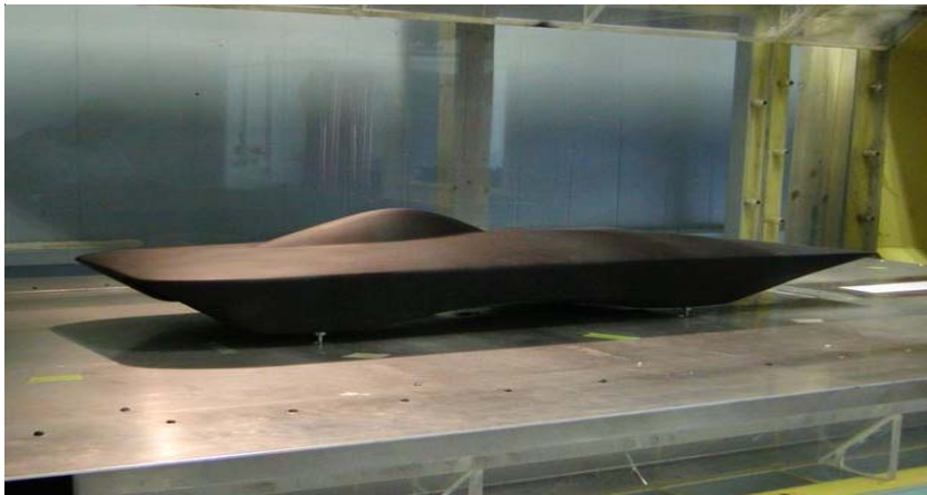
Figure 2. The experimental model of the Sunseeker sits in the test section of the WMU wind tunnel.
