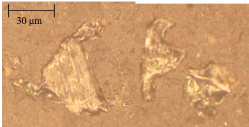
Figure 8: NC-AP Sample Showing Voids (a right, b left).
