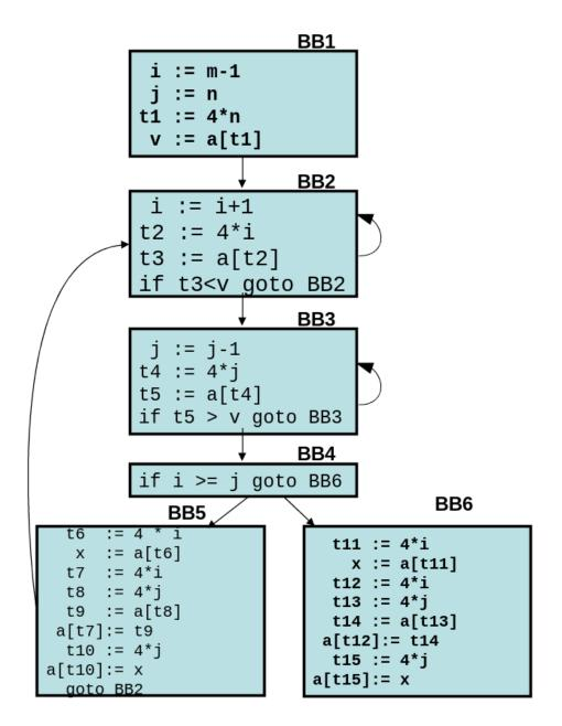
Figure 2.1: An example control flow graph
