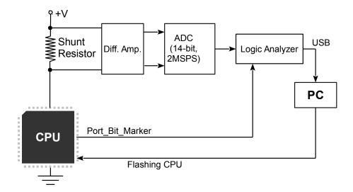
Figure 3.1: Capture setup
