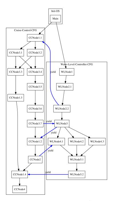
Figure 3.4: CFG of the system with two tasks (one instance)
