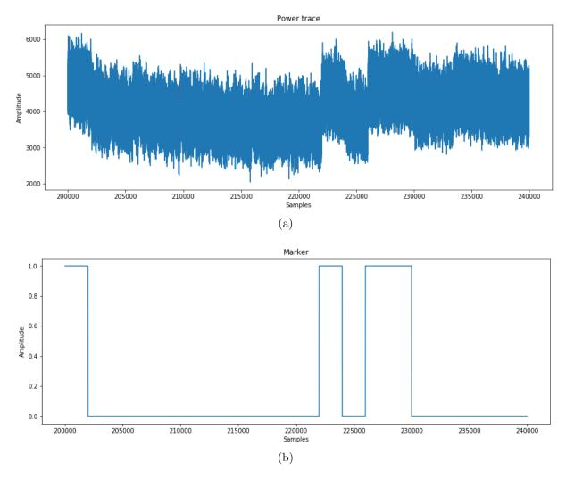
Figure 3.2: Powertrace with marker
