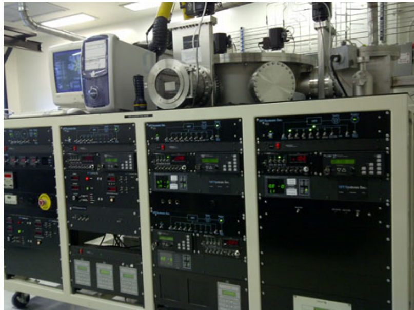
Figure 2-6: MVSystems multi-chamber PECVD system used for nc-Si and \text{SiN}_x deposition.
