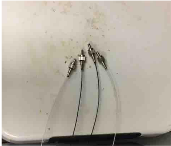
Fig. 11. Image of the input legs of 2 couplers with epoxy curing on top of the hot plate at 100° C. Some connectors still have the tip of the fiber that was later cut for polishing.
